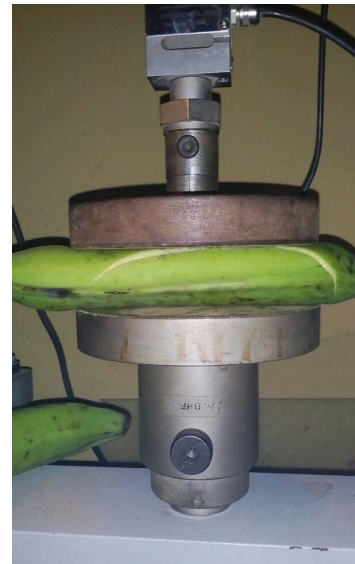
Fig. 1. Plantain finger undergoing quasi compression testing
