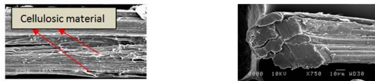
(b) China-rose stem fibre with X 1000 and cross section view of fibre (X 750 magnification)
