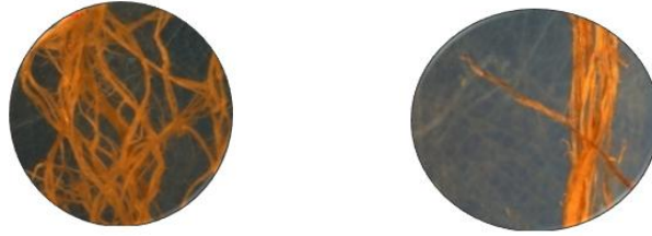
Fig 4. Microscopic structure of china-rose fibres
