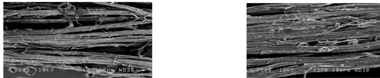
(a) SEM of China-rose fibre (China-rose bundle fibres with X 90 and X 270 magnification)
