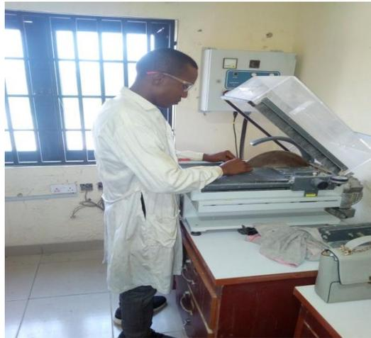
**Plate 1. Thin Section Preparation**
