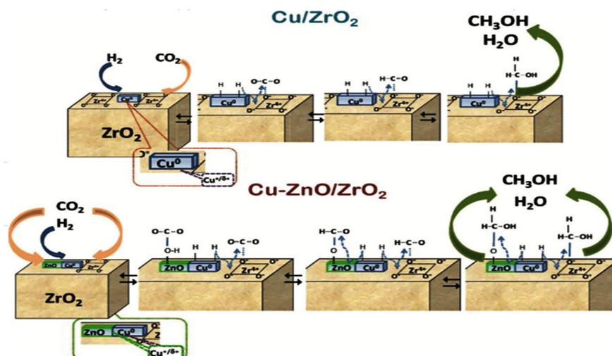
**Figure 7.** Heterogeneous catalytic process for conversion of  $\text{CO}_2$  to methanol using  $\text{Cu}/\text{ZrO}_2$  and  $\text{Cu-ZnO}/\text{ZrO}_2$  (adopted from [20]).
