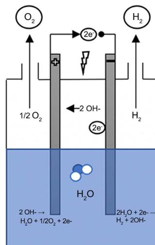
**Figure 4.** An electrolyzer (Re-produced from [16]).
