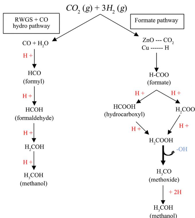
**Figure 8.** Pathways of methanol production from  $\text{CO}_2$  hydrogenation over Cu-based catalysts (Reproduced from [1]).
