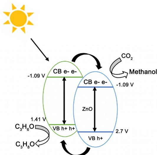
**Figure 5.** Schematic of photocatalytic reduction of  $\text{CO}_2$  system [24].
