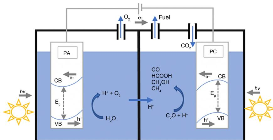
**Figure 6.** Photoelectrocatalytic cell for CO<sub>2</sub> reduction (reproduced from [26]).
