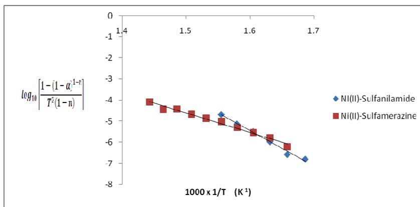
Fig. 8. Coats Redfern plot for second stage of decomposition for both the complexes
