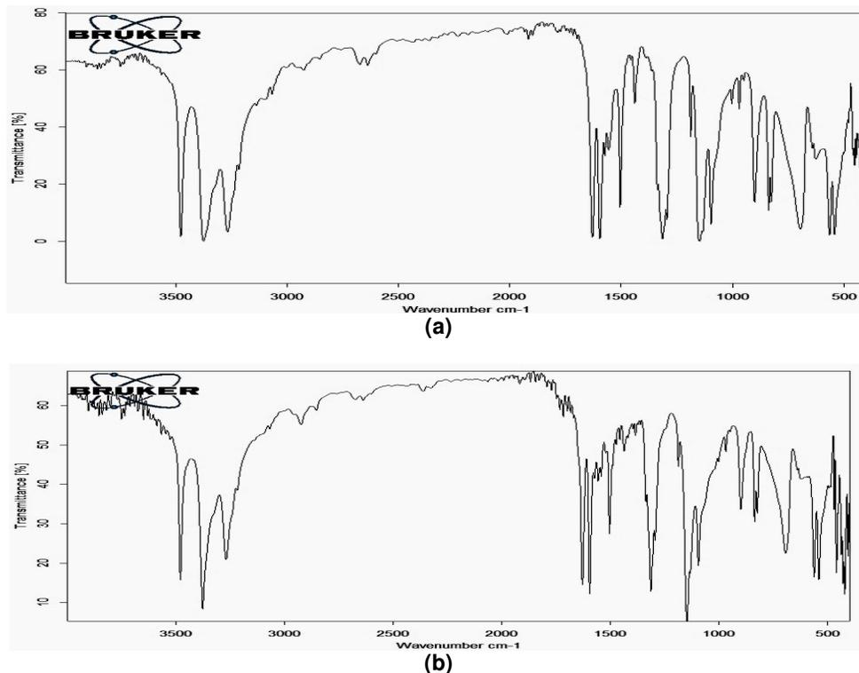
Fig. 4. Experimental FT-IR spectra of (a) Sulfanilamide, (b) Ni(II)-Sulfanilamide complex
