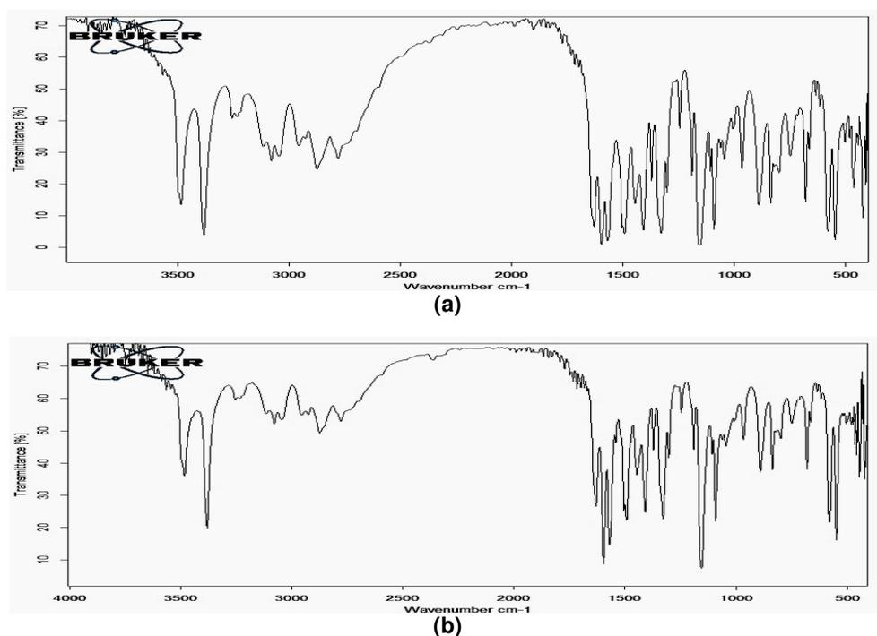
**Fig. 5. Experimental FT-IR spectra of (a) Sulfamerazine and (b) Ni(II)-Sulfamerazine complex**
