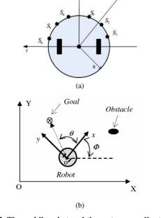
Figure 2. The mobile robot and the system coordinate. XOY is the world coordinate and XOY is the robot coordinate. Goal and Obstacle are marked respectively.
