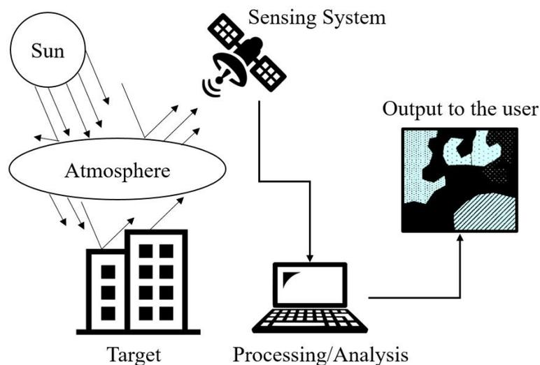
**Fig. 2. Components of a remote sensing system**
