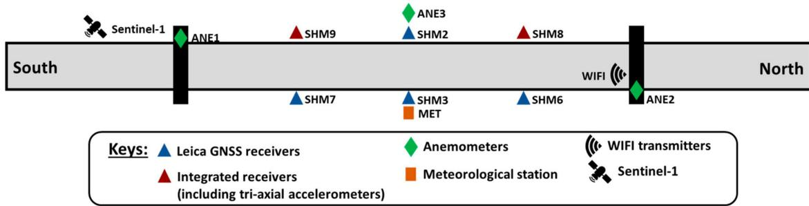
Fig. 14. GeoSHM sensor system of the FRB [46]
