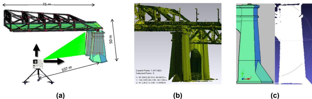
Fig. 17. (a) Layout of the scanning problem, (b) Data acquisition, and (c) BrIM results vs. scanned results [47]
