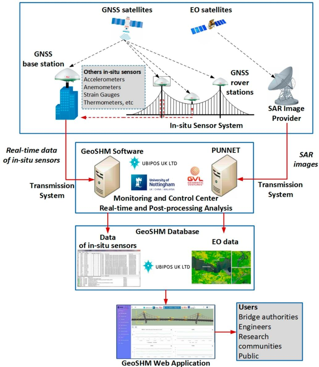
Fig. 15. General structure of the GeoSHM system [46]
