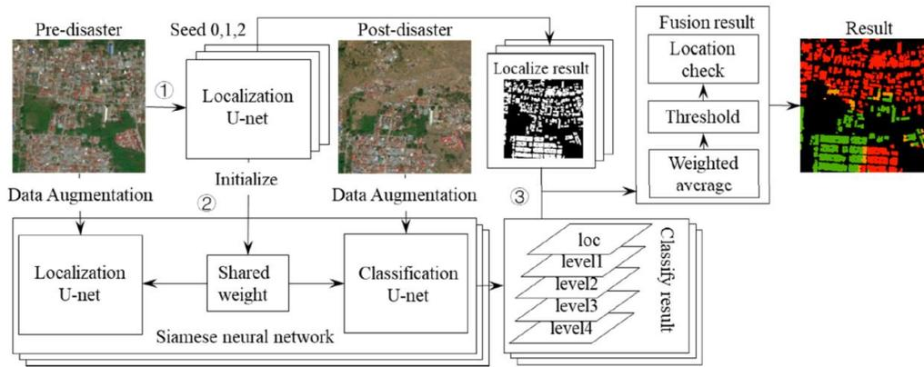
**Fig. 9. The proposed building damage detection methodology integrated with remote sensing [42]**
