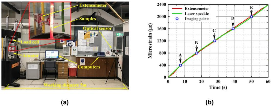
Fig. 18. (a) Laboratory test of the laser speckle imaging sensor, and (b) Validation of LSIS results [48]
