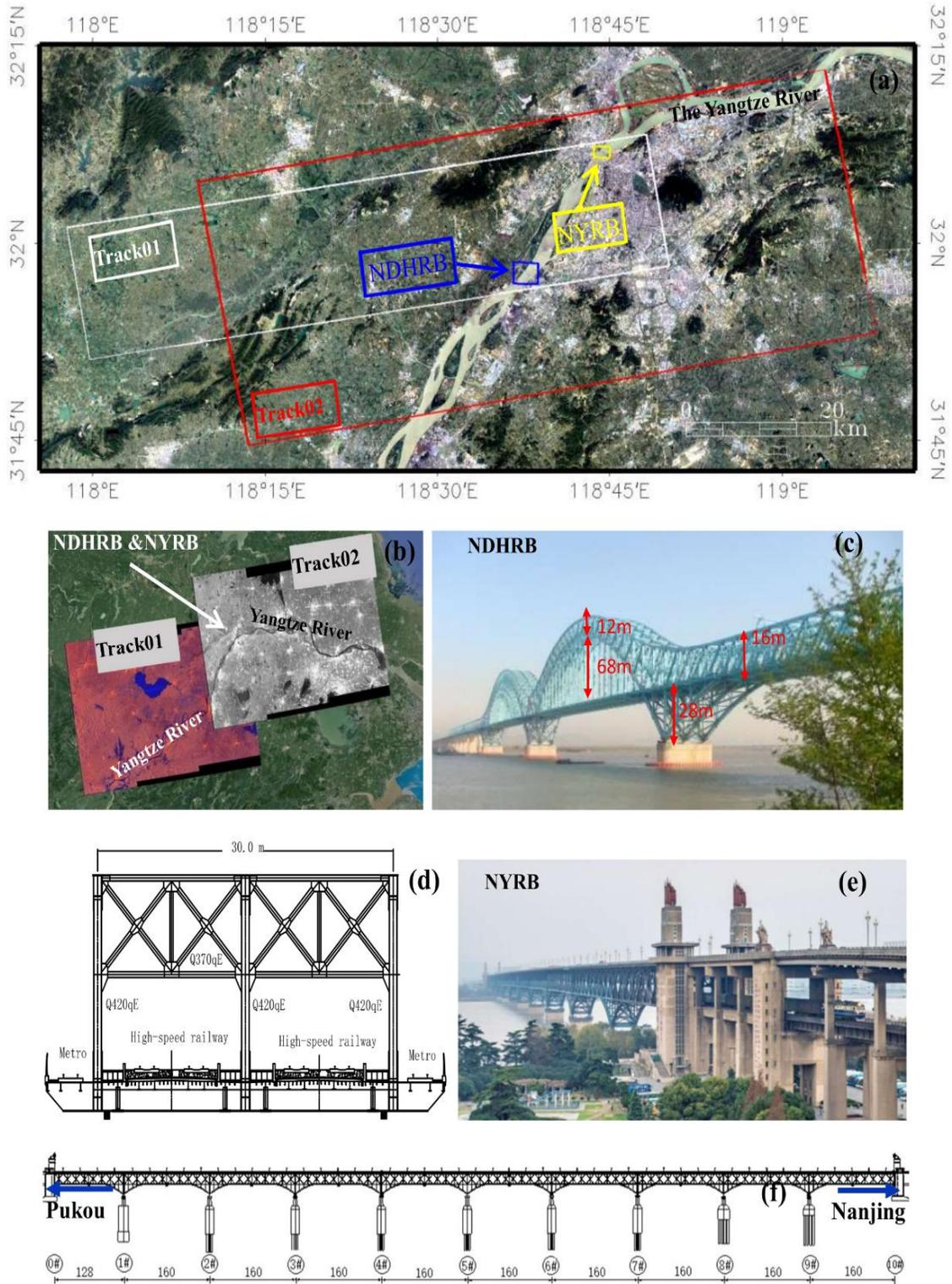
Fig. 11. (a) SAR image presenting the location of bridges and burst coverage, (b) Tracks footprint, (c) NDHRB, (d) NDHRB cross-section, (e) NYRB, and (f) NYRB layout [43]
