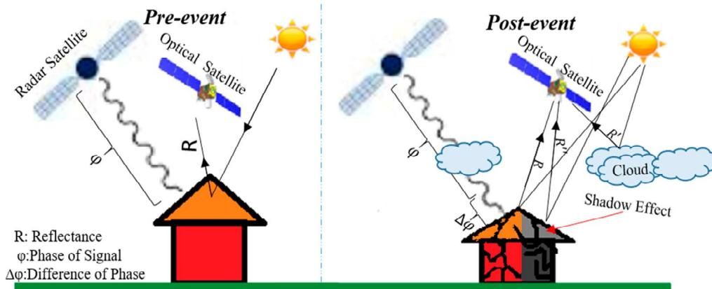
Fig. 19. The ability of radar data for detecting damaged areas under cloud and shadow conditions [49]
