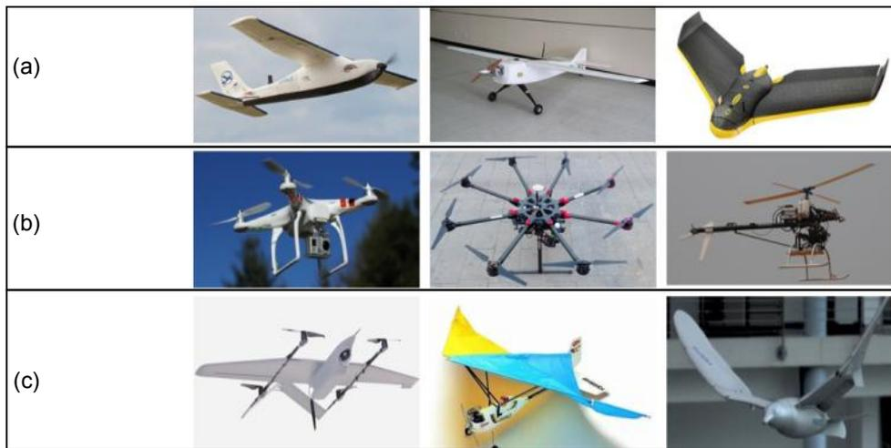
**Fig. 20. A number of UASs for remote sensing: (a) Fixed-wing UAS, (b) Rotary-wing UASs and unmanned helicopters, and (c) Hybrid UAVs, umbrella-UASs, and bionic-UASs [51]**
